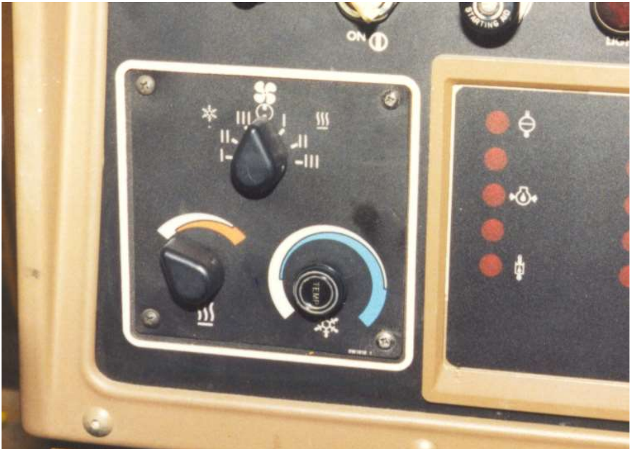
Thermostat in location on dash control panel.
