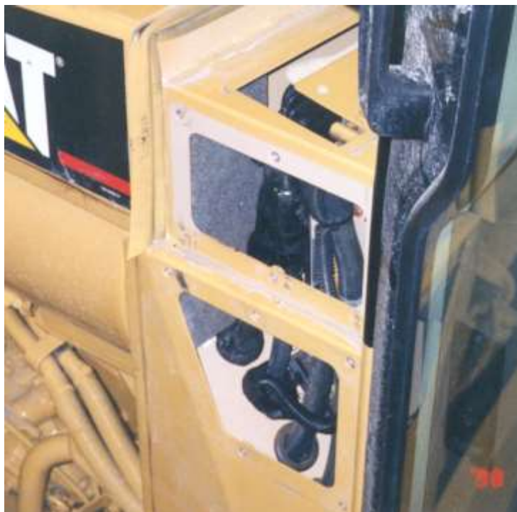
Evaporator assembly showing hoses.
