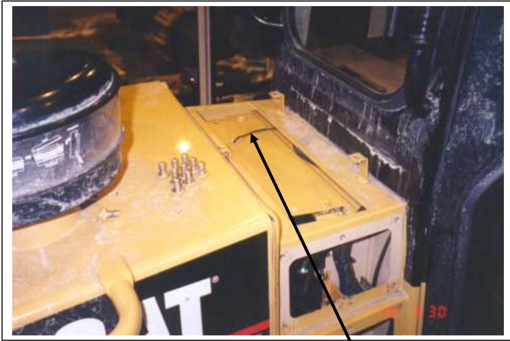
Evaporator cover in place with thermostat.
